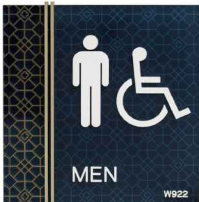
Thermoform Sign • Subsurface Printed Pattern & Floodcoat • Right Side: Integral Text & Domed Grade 2 Braille Painted White with Super Matte Finish • Left Side: Etched & Filled Pattern with Museum Polished Face • Routed Channels to Receive Metal Accent Bars • Square Corners
